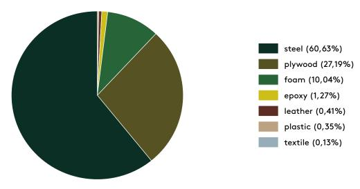
Based on: Frame epoxy | 8 kg
