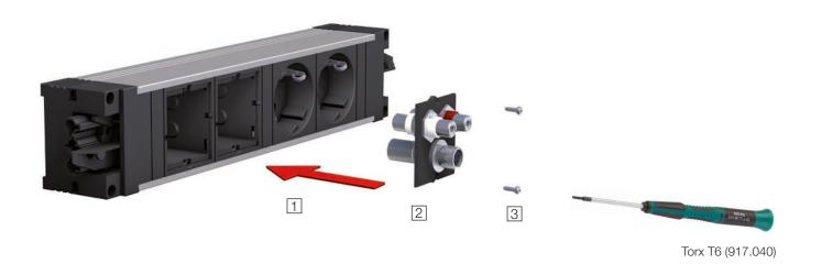
The empty built-in frame 1 of Bachmann FACILITY SOLUTIONS accommodates the custom modules 2, which are fixed in place with two Torx screws. The custom modules can be easily exchanged by loosening the screws.
