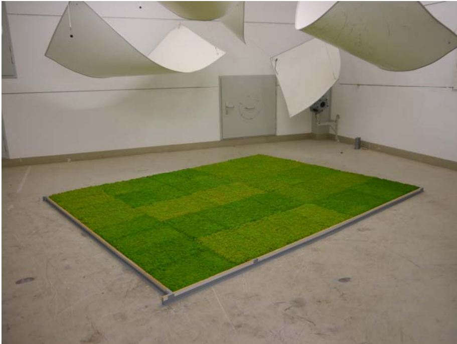
Figure B.1. Arrangement of the test object on the floor of the reverberation room.
